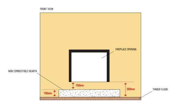
For installations where a combustible floor is situated in front of the Stuv 21 a non combustibe hearth (floor protector) is required.
